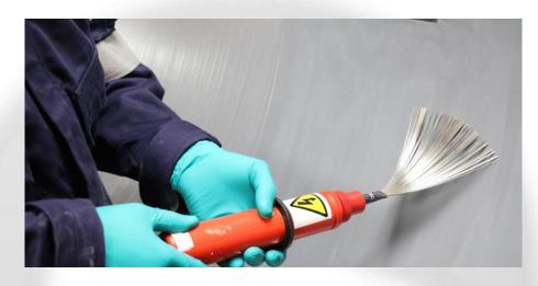
Holidays tests work on the concept of electrical conductivity. Metal substrates are excellent conductors of electricity, and therefore allow current to flow through them. On the other hand, many coatings are poor conductors of electricity and resist the flow of electricity. Using this principle, holiday tests use instruments to locate flaws in anticorrosive paints and coatings.
