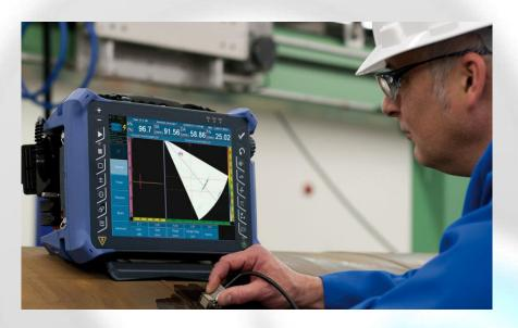
Phased array systems pulse and receive from multiple elements of an array. These elements are pulsed in such a way as to cause multiple beam components to combine with each other and form a single wave front traveling in the desired direction. Similarly, the receiver function combines the input from multiple elements into a single presentation.
